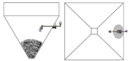
Figure 2: volcan Location Schematics (side and top views)
